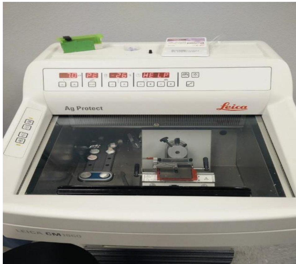
Figure 72 Cryotome used to slice specimens
