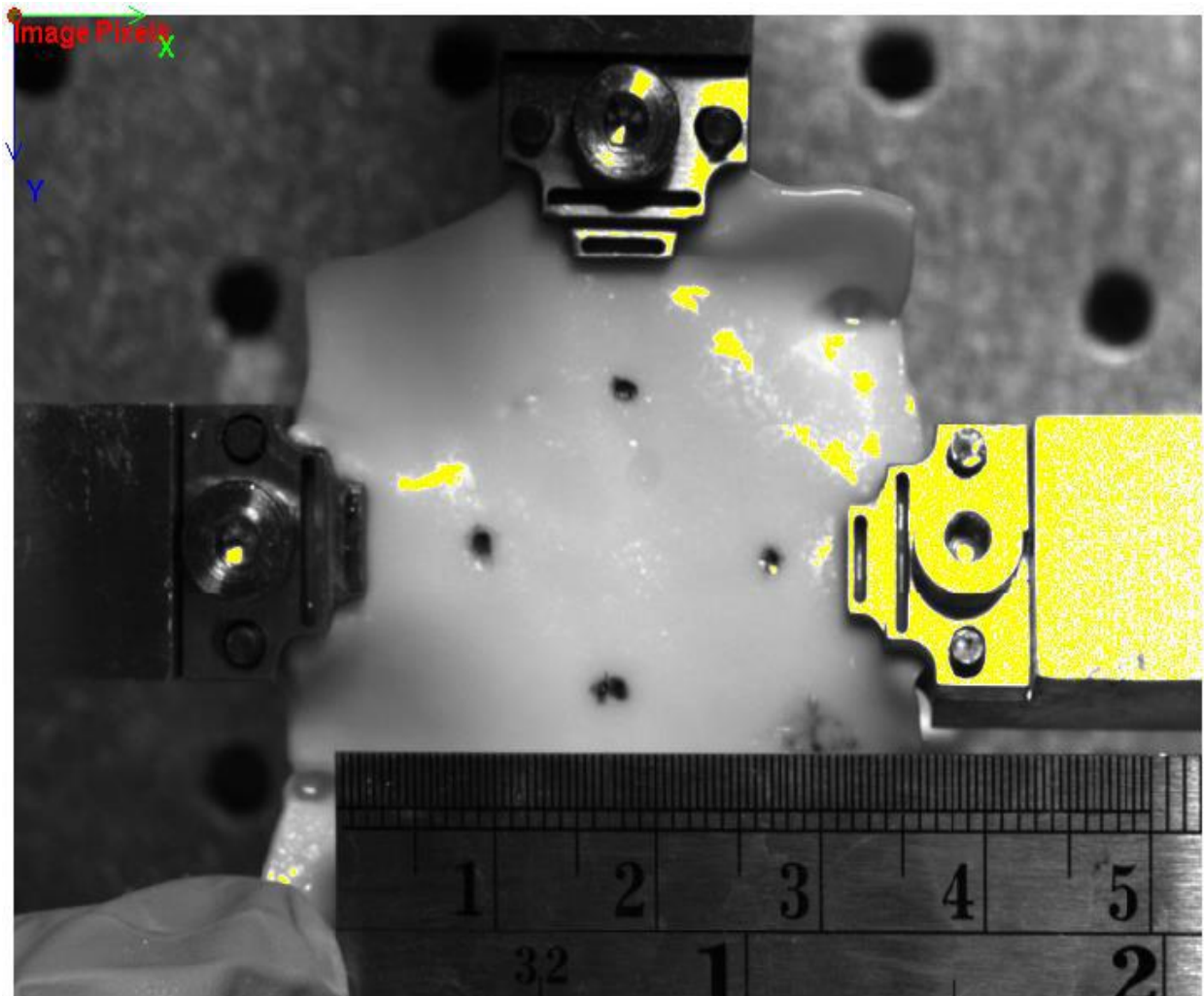
Figure 62 TestResources Biaxial Testing machine with a specimen mounted where the vertical direction is the longitudinal orientation and the horizontal direction is the circumferential orientation.
